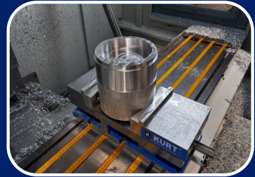
Canard Housing in CNC Setup
